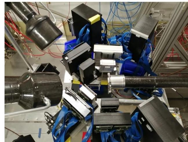
i-TED array prototype with four large Compton cameras under commissioning at CERN n\_TOF EAR1 in 2021 (HYMNS-ERC).
