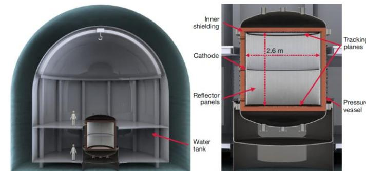
Conceptual design of a tonne-scale NEXT experiment for neutrinoless double-beta decay searches, installed inside a water tank (left), and detail of the internal structures of the detector (right)
