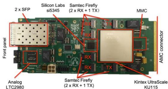
Picture of the Compact Processing Module version 2 of the ATLAS Tile Calorimeter with the main components labelled.
