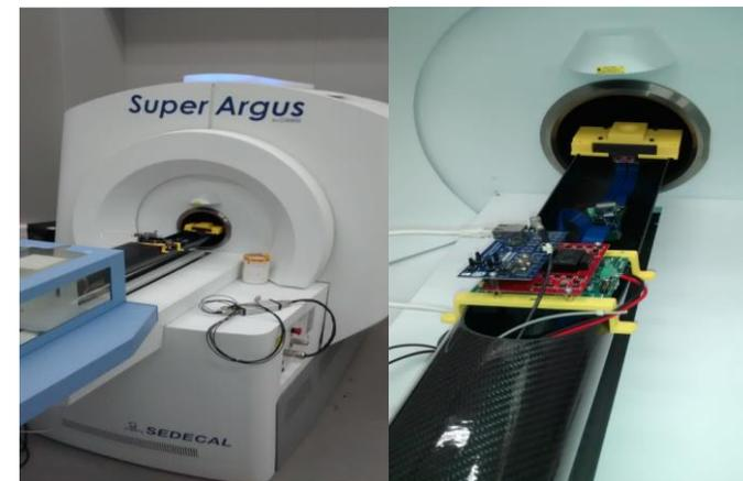
PROScRiPT probe being tested in the Super Argus 4R PET scanner (left) and detail of the probe (right).
