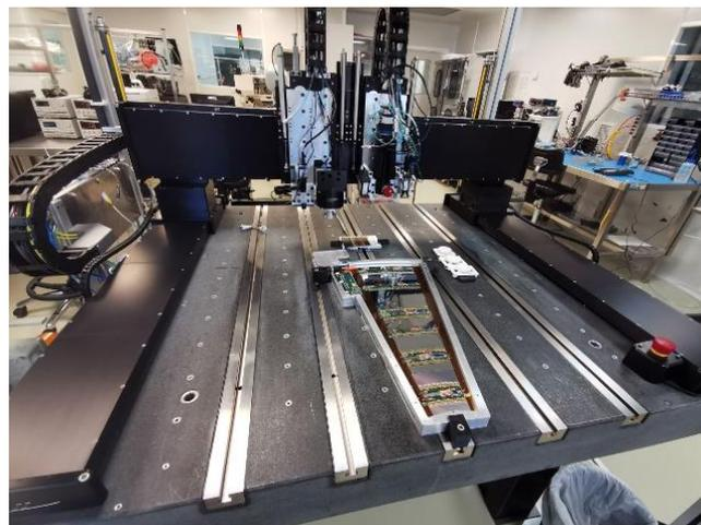
Petal core of the ATLAS Inner Tracker being loaded with petals in the gantry of IFIC's clean room.
