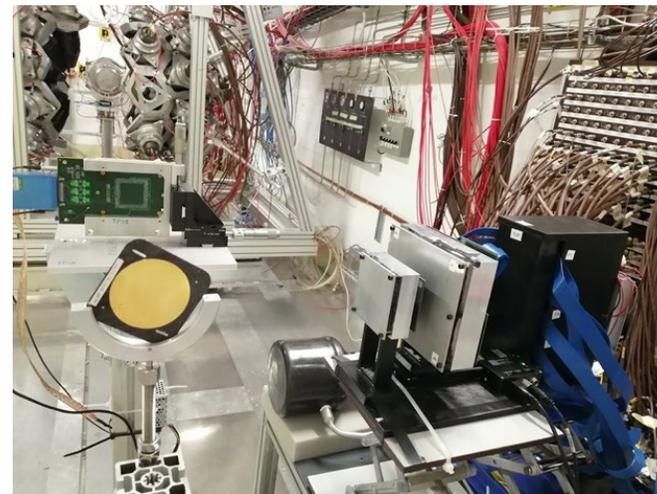
Caption: One of the four high-efficiency i-TED Compton modules (right) installed in the EAR1 experimental room of the CERN n\_TOF laboratory
