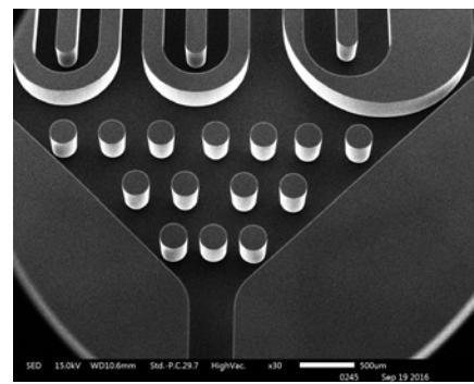
Schematic representation of micro-channel cooling for silicon sensors and detail of the cooling circuit implemented in a silicon sensor
