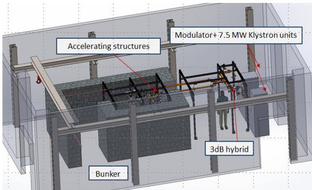
Scheme of the IFIC High-Gradient RF Laboratory.
