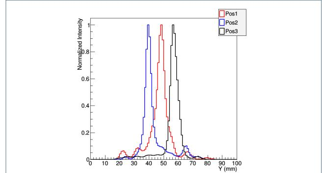
Profiles of the images obtained with 4.4 MeV gamma rays obtained with the telescope in three different positions with respect to the target, separated 10 mm. The telescope response was also characterized with different geometries, placing the detectors at different distances to one another and from the source. The results were compared to simulations with GATE, with very good agreement.
