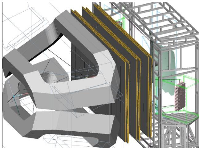
Schematic view of the upgraded LHCb central tracker (SciFi), downstream of the dipole magnet (on the left).
