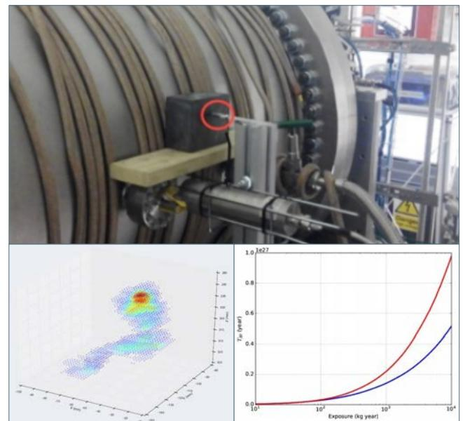
Above:  $^{22}\text{Na}$  source deployed in the lateral port of NEW. Down (left): reconstructed electron track in NEW. Down (right): NEXT-100 sensitivity to the  $\text{bb}0n$  half-life according to arXiv:1511.09246 (blue) and to the improvements based on DNNs (red).
