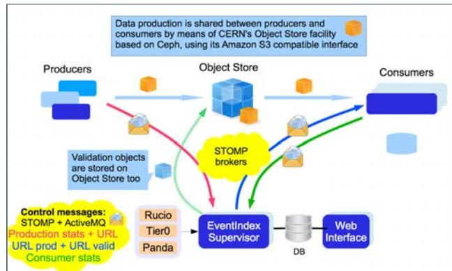
Flow diagram of the Event Index prototype, involving the components Producer-Supervisor-Consumer which are responsibility of the IFIC team. The group is working in the ATLAS Event Index Project updated with the new features developed during 2016: web interface, Object Store, etc.
