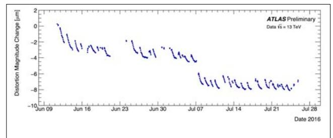
Bowing magnitude of the IBL staves during the 2016 ATLAS data taking. Each point corresponds to data accumulated during 100 minutes.
