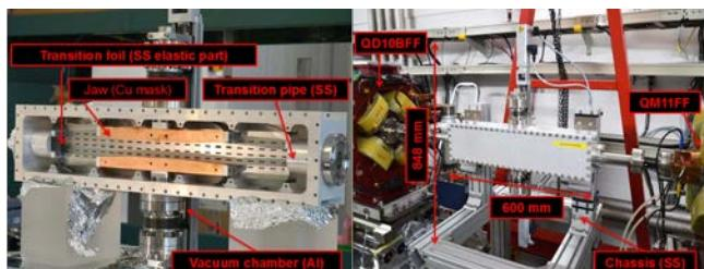
Movable collimator installed in ATF2
