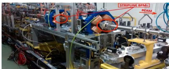
Prototype stripline BPMs installed in the CLIC Two Beam Module
