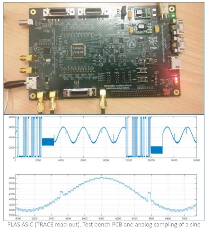
PLAS ASIC (TRACE read-out). Test bench PCB and analog sampling of a sine wave.
