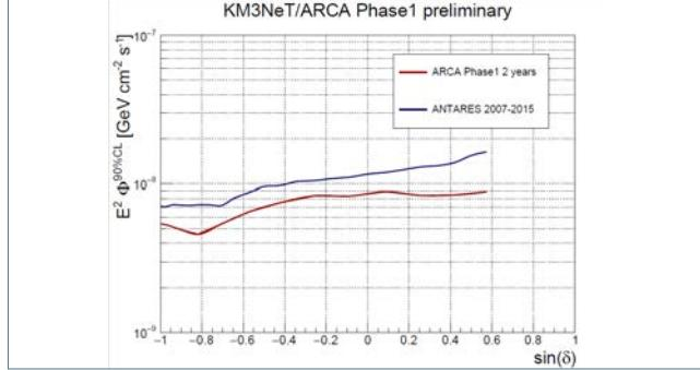
Up: Connection of one of the lines of KM3NeT in the deep sea. Down: Comparison of the sensitivity for point sources of two years of ARCA Phase 1 and the present limits of ANTARES.
