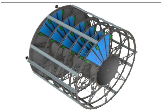
Partially loaded global structure of one of the two endcaps that form the silicon strip detector of the HL-LHC ATLAS inner tracker (ITk). This is the design proposed by our group and chosen as the baseline.
