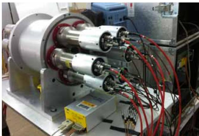
The total absorption spectrometer designed by IFIC and employed in the experiments.
