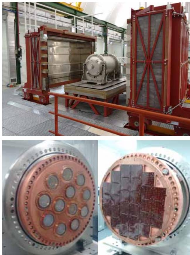
Pictures of NEXT-White (NEW) installation at the LSC during 2015. Up: pressure vessel and shielding. Left: energy plane. Right: tracking plane.
