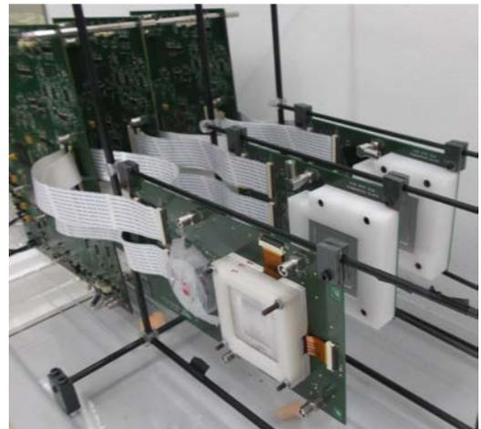
Compton telescope composed of three  $\text{LaBr}_3$  detectors connected to the readout electronics.
