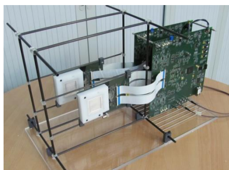
Compton telescope composed of two LaBr3 detectors connected to the readout electronics
